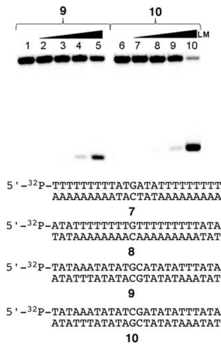
Figure 7. Alkylation of palindromic DNA sequences by activated leinamycin. The palindromic duplexes 5'- 32 P-TATAAATATATGCATATATTTATA (9) and 5'- 32 P-TATAAATATATCGATATATTTATA (10) were incubated with leinamycin and 2-mercaptoethanol at 30 °C for 23 h in HEPES buffer (50 mM, pH of 7) DETAPAC (5 mM), followed by Maxam–Gilbert workup and separation of the resulting DNA fragments on a 20% denaturing polyacrylamide gel. Reactions analyzed in lanes 1–5 contained duplex 9, while lanes 6–10 contained duplex 10. Reactions analyzed in lanes 1 and 6 contained DNA treated with 2-mercaptoethanol (5 mM, no leinamycin); lanes 2 and 7, contained DNA treated with leinamycin (10 \mu\text{M} ) and 2-mercaptoethanol (5 \mu\text{M} ); lanes 3 and 8, contained DNA treated with leinamycin (100 \mu\text{M} ) and 2-mercaptoethanol (50 \mu\text{M} ); lanes 4 and 9, contained DNA treated with leinamycin (1 mM) and 2-mercaptoethanol (0.5 mM); lanes 5 and 10 contained DNA treated with leinamycin (10 mM) and 2-mercaptoethanol (5 mM).
